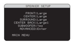
The SPEAKER SETUP menu is used to configure the RSX-1067 for use with your specific loudspeakers and to determine the bass management configuration as described in the previous overview. The menu is accessed from the MAIN menu.
